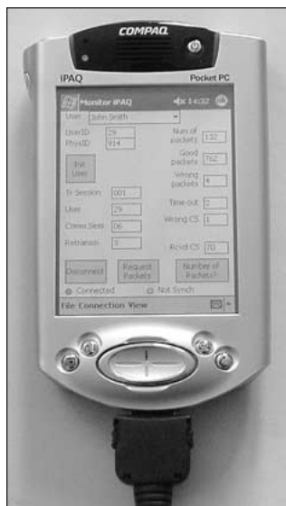
Fig. 3. Monitoring application running on mobile gateway (MOGUL).
