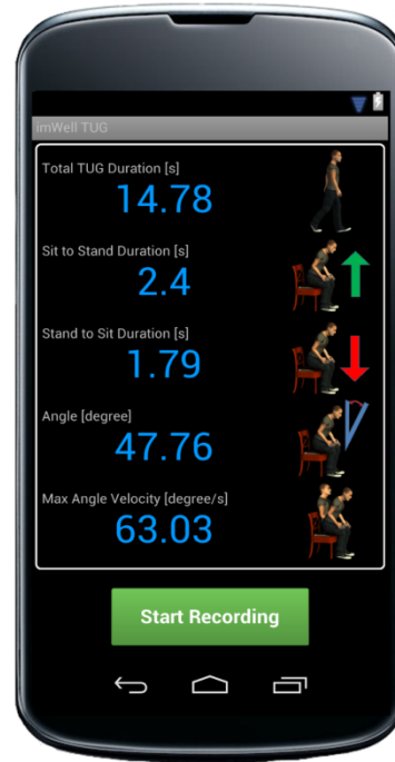
Figure 5. sTUG: Smartphone TUG Android application screen displaying the parameters of the TUG test.
