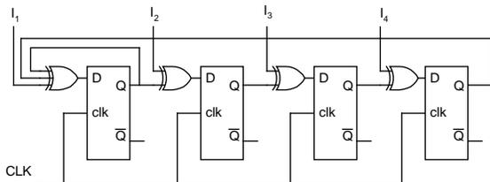
**Figure 2 An implementation of a 4-bit MISR.**
